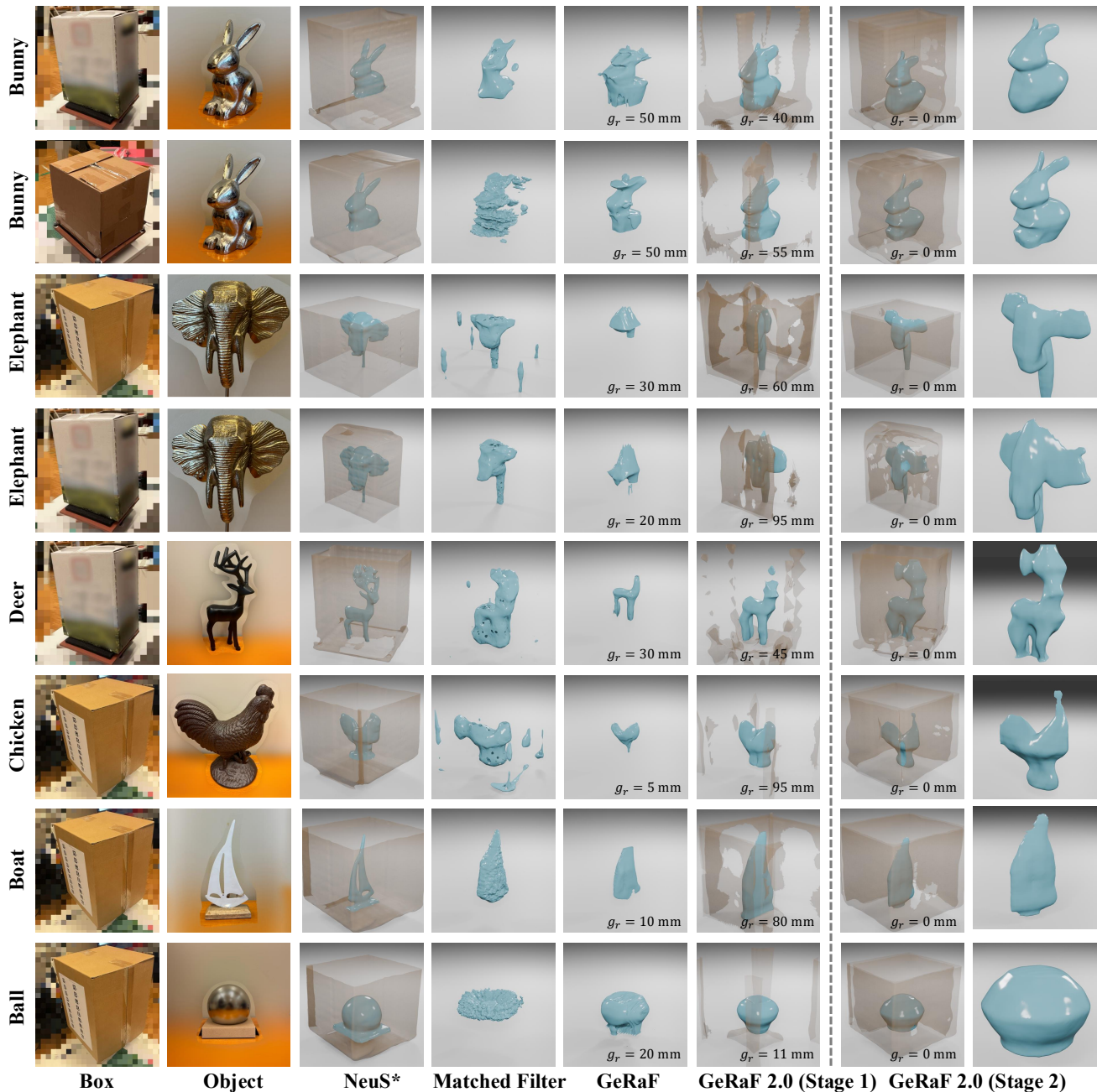
Figure 8. Qualitative results between vision-based NeuS [46], point cloud-based reconstruction using matched filter, non-line-of-sight reconstruction with GeRaF [29], and GeRaF 2.0 in Stage 1 and Stage 2. *For NeuS, the object and box are captured separately visualized together via post-processing. For GeRaF and Stage 1, the surface level g_r is manually selected (indicated in the visualization).
